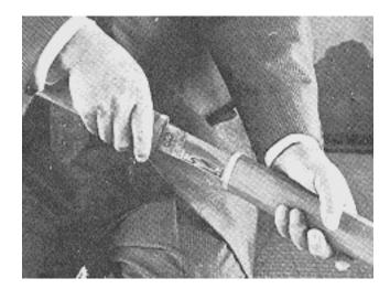
**3.** To remove the hilt, hold its end with the left hand on the side where the back of the blade is fit, and keep the blade in a slightly angled upright position. Use the right fist to hit the left wrist lightly a few times. When the tang (nakago) becomes slightly loosened in the hilt, repeat until the tang comes out of the hilt by itself. When there is enough room to grasp the tang, the blade may be pulled out of the hilt by the right hand.
