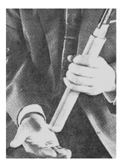
Then, pass the blade to the right hand, pick up the scabbard and slide the blade into it observing the manner described in Section II. Needless to say, the other parts like spacers and sword guards of fully mounted swords must also be returned to their respective places before the hilt is put on the tang.
